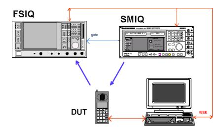
Fig. 1: Minimum equipment configuration
