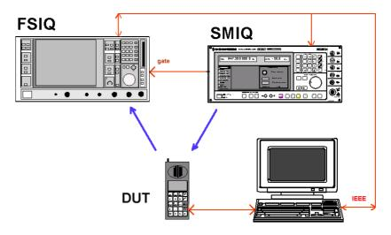
Fig. 6: Signal paths for spectral measurements
