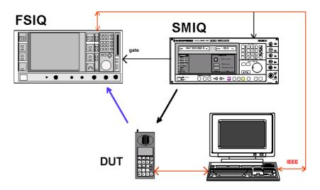
Fig. 2: Signal paths for TX measurements
