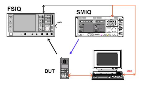
Fig. 10: Signal paths for bit error measurement with decoded bits returned
