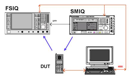
Fig. 11: Signal paths for bit error measurement with RF loopback
